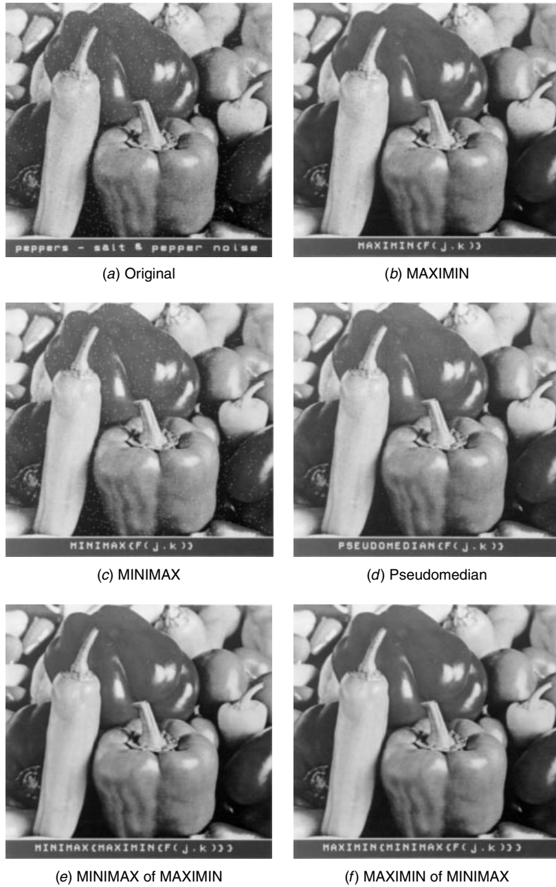
FIGURE 10.3-15. 5 \times 5 plus-shape MINIMAX, MAXIMIN, and pseudomedian filtering on the noisy test images.
